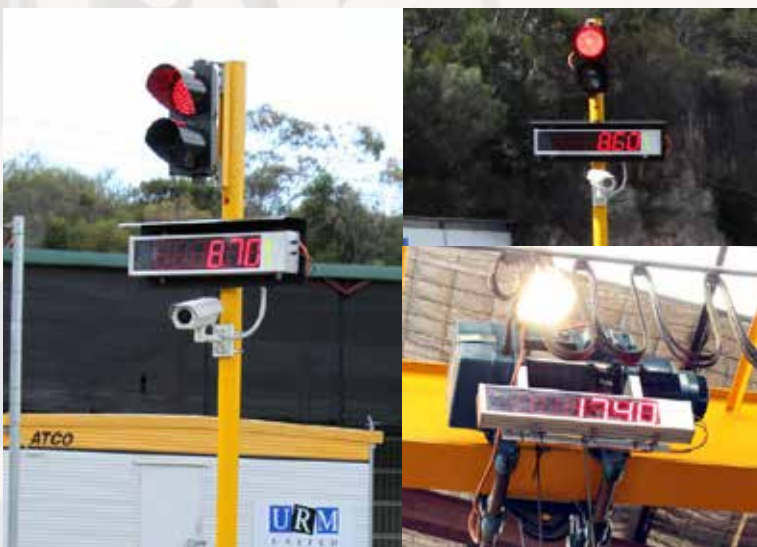
The GS120 Indicator in Action On Weighbridges & Overhead Cranes
