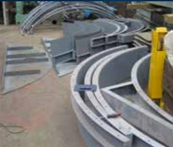
Section Of Bolted Carbon Steel Tanks
